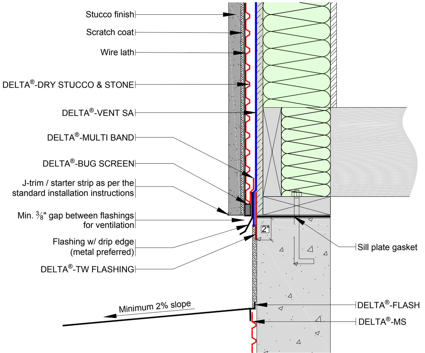
\*\*For proper performance of DELTA®-DRY ensure top and bottom remain open to allow ventilation and drainage\*\*
