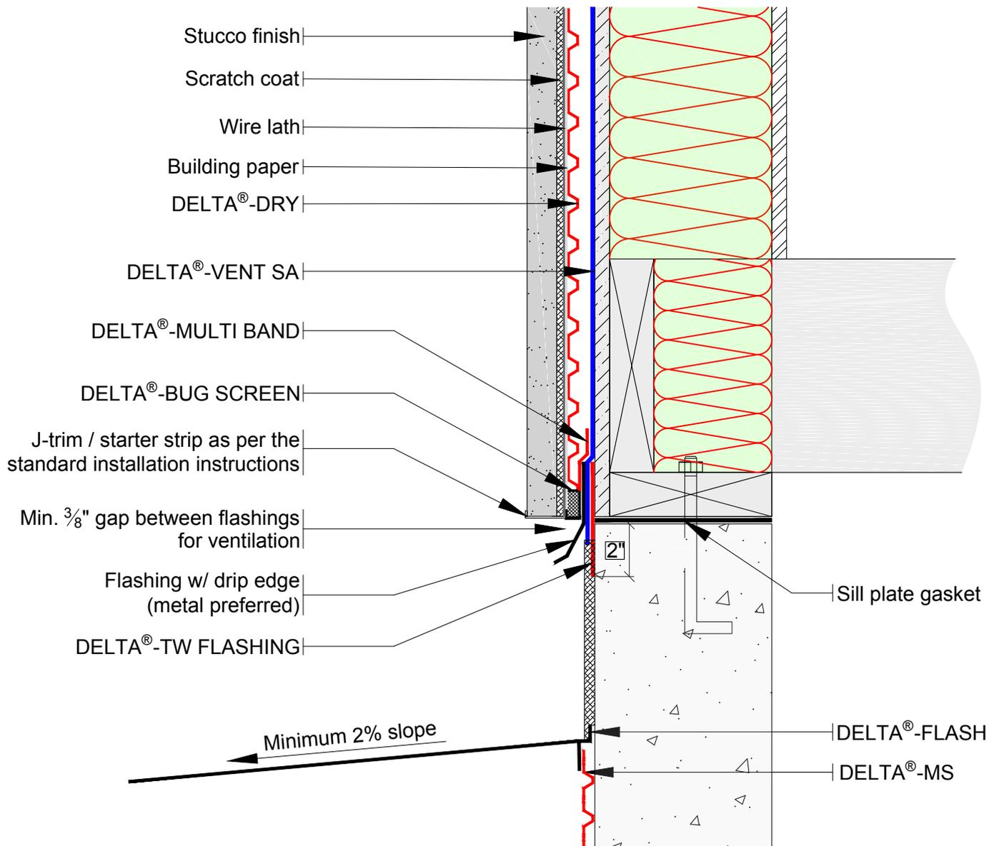
\*\*For proper performance of DELTA®-DRY ensure top and bottom remain open to allow ventilation and drainage\*\*
