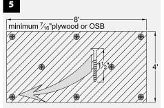
8 Tapcon® screws per 1, 4'x8' sheet of plywood or OSB
