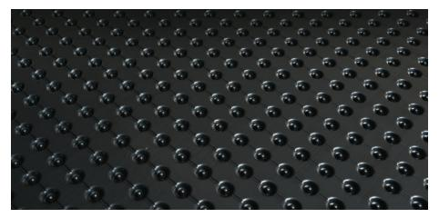
In homes, laminate flooring and its underpad can by placed directly over Platon as a floating floor. For other floor finishes, plywood or OSB sheets (11mm or 7/16" minimum thickness) are laid as a secured subfloor over the Platon and fastened to the concrete floor with concrete screws or masonry nails.
